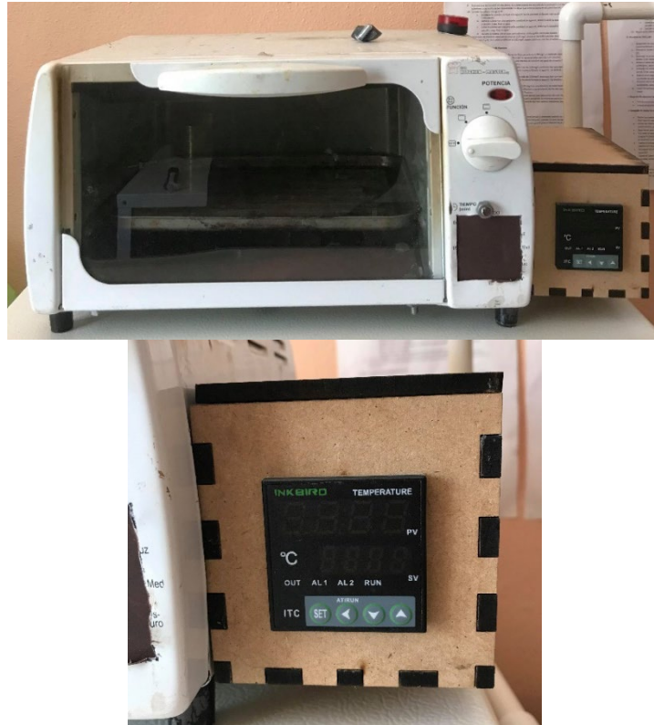
Figure 4.1.1.2 - Top: PID oven system. Bottom: PID controller unit
