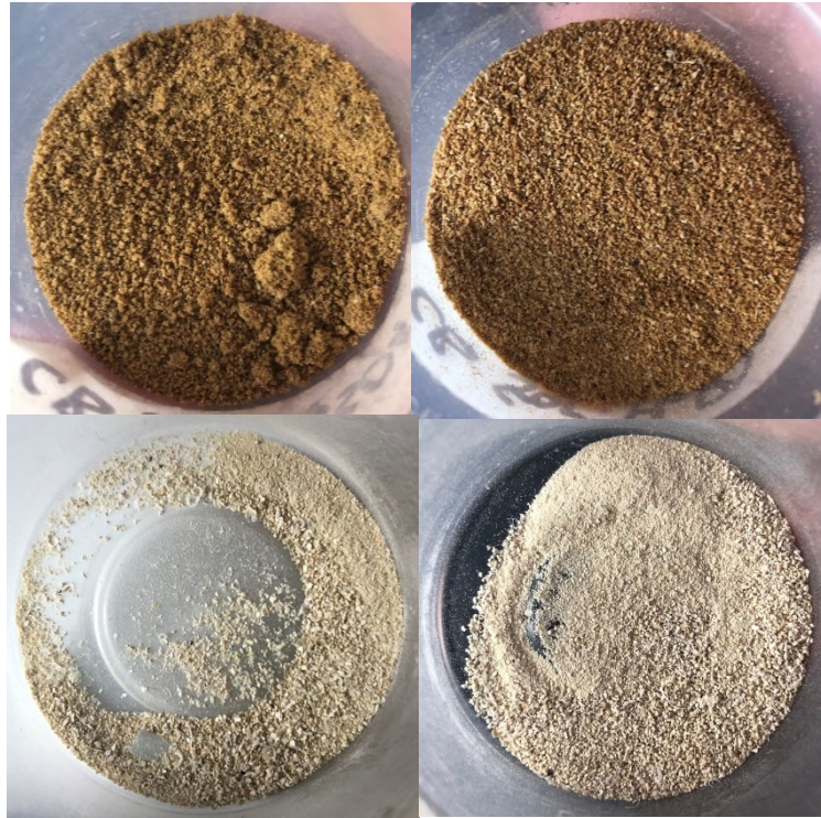
Figure 6.1.3.6 - Top left: H 2 SO 4 CAB. Top right: H 3 PO 4 CAB. Bottom left: KOH CAB. Bottom right: NaOH CAB.
