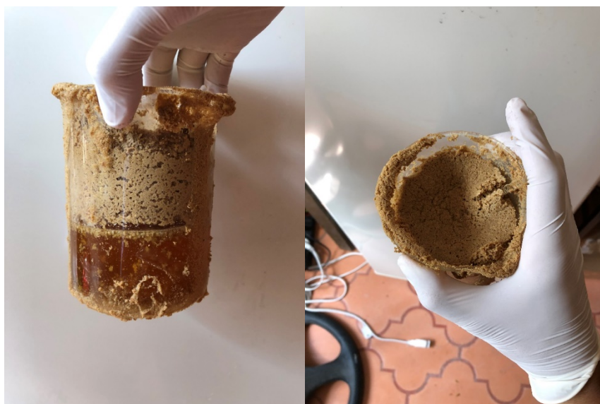
Figure 6.1.3.1 - Bone meal slurry after soaking for 24 h in 13 wt. % NaOCl. Left: Side view. Right: Top view.
