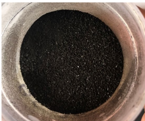
Figure 6.2.3.1 - Dry RBC sieved through US standard # 30 mesh for use in batch test 2
