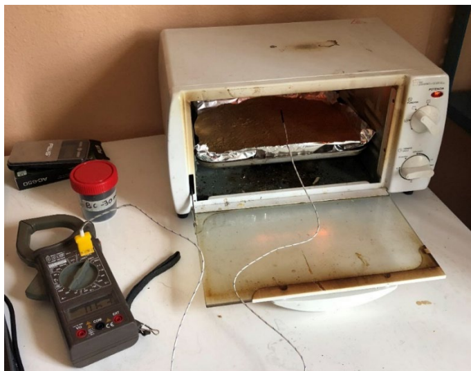
Figure 8.1.1.1 - Toaster oven with thermocouple setup used to dry samples
