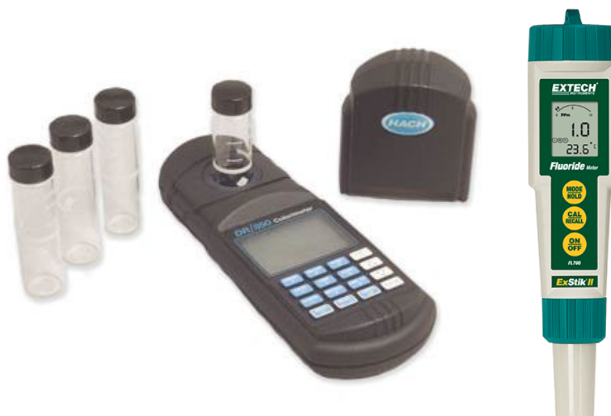
Figure 4.1.4.1 - Left: Hach DR/890 portable colourimeter with sample beakers [100]. Right: Extech Instruments FL700 fluoride ion selective electrode probe [118].
