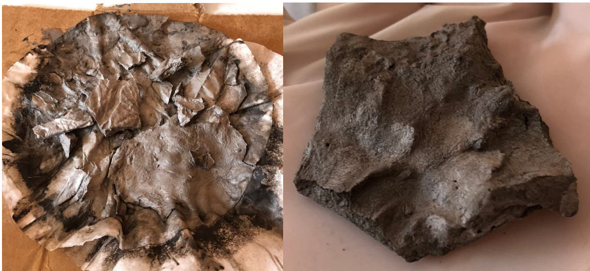
Figure 6.1.4.1 - Left: dry CABc cake on filter paper. Right: Close-up of CABc cake piece.
