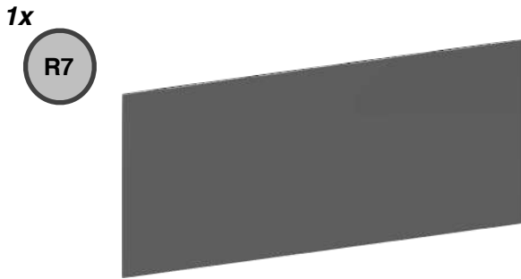
2-3mm thick sheet metal. Cut a piece 39x59cm.
