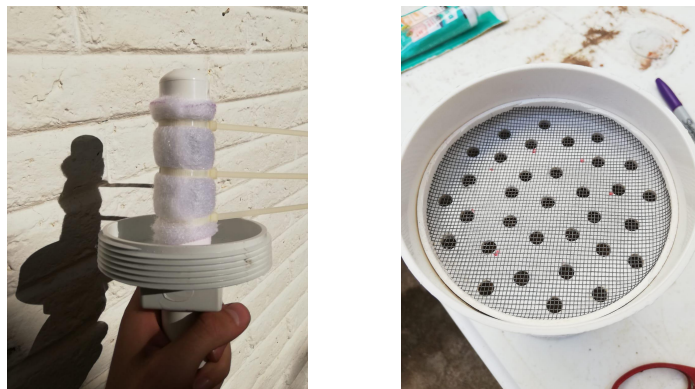
Figure 3: From left to right: top/inlet of the column; perforated base plate of the column
